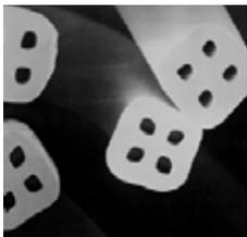
→ Antron® carpet fiber uses hollow filament shapes which minimize the soil trapping area of the fiber and the appearance of soil. The hole(s) refract and diffuse light to hide the effects of soil, while specially designed outer surfaces make it easier for soil to be released during cleaning.
